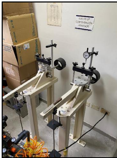
Figure 1. Consolidation Equipment at the Soil Mechanics Lab.
