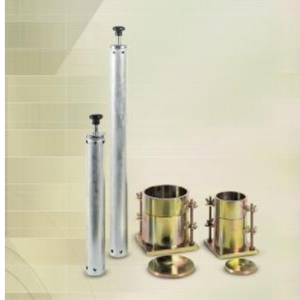
Figure 1. Compaction Test Equipment. Controls Group.
