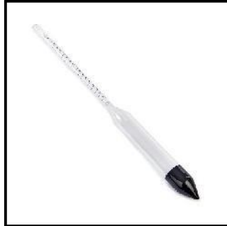
Figure 3. Hydrometer used to measure the Soil Particles falling. VintEssensial.
